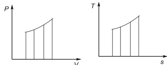
Area under curve on P-V represents work when projected on volume axis for closed system
